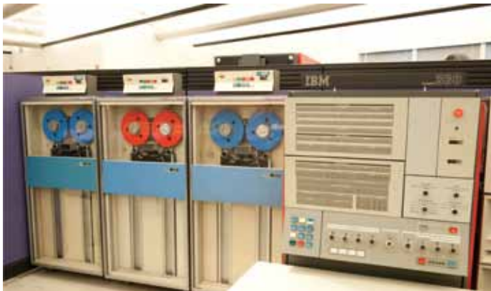
Figure 4: A relic from the enterprise computing era: the IBM System 360 mainframe, sold 1964 to 1978.
